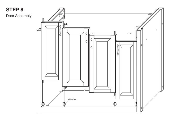
Slide top front brace down into position to secure doors. Fasten with 1 3/4" bolts and nuts as shown.
