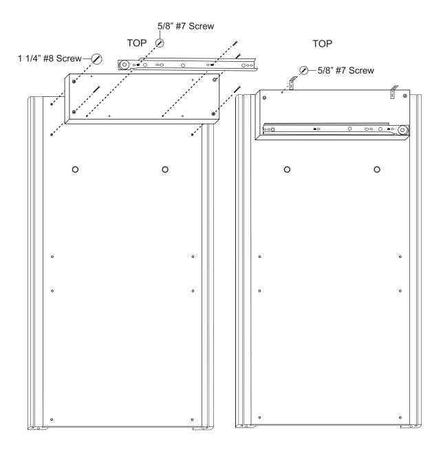
A. Lay Back Panel flat on a smooth surface with holes up.
