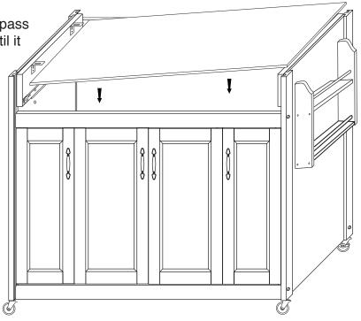
A. Tap 1" pins into the 4 sets of holes in the Back Panel. B. Just above the Bottom shelf on the inside of the Bottom Front Brace there are two sets of holes. Tap 1" pins into these holes.
