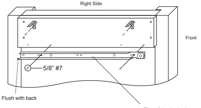
Note: Glide holes sometimes change, just make sure the cabinet glides are flush with the back of the glide supports & pilot holes will line up only 2 holes are used! The glides look almost alike; however, they are stamped CR for cabinet right and CL for cabinet left.
