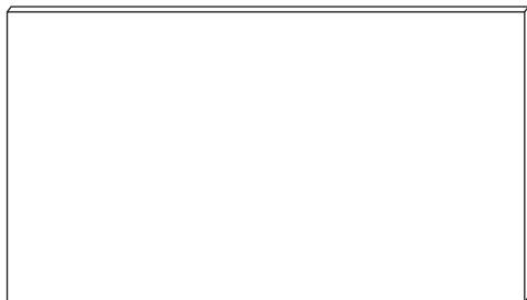
Drawer Bottom (1) P/N DBOT-1468 14 5/8" x 14 5/8" x 5/32"
