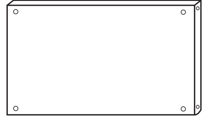
Top Side Braces (2) P/N B-1469/TS 13" x 7.75" x 3/4"
