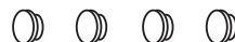
(4) 3/4" Wooden Disks Fit in Nut Access Holes in the Bottom Support Brace (Identical)
